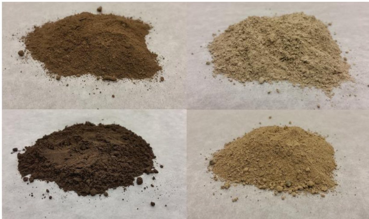
Figure 1. Figure 1. Unprepared samples counterclockwise from top left - 132, 164, 230, and 497 (control). Each sample has different physical properties, such as color and texture, determined by the mineralogical and biochemical composition of the sediments.
