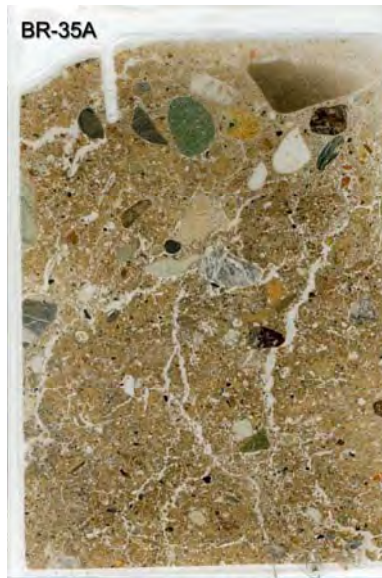
Macro scan of large thin section BR-35A. Note the overall lighter color of this material, suggesting an increase in natural sediment as one approaches the base of the structure.
