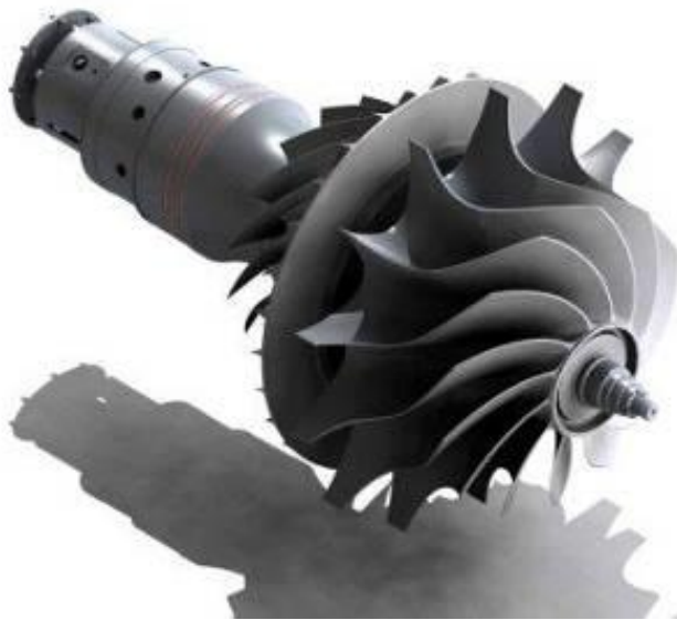
Figure 1: Compressor and rotor in an integral design with an overhung configuration
