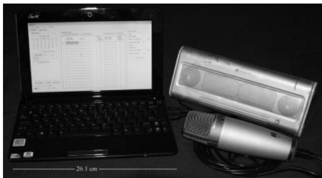
**Figure 1.** Photograph of netbook computer, microphone, and 20-W speaker used as an acoustic wildlife survey device in Idaho, USA, 2010.
