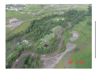
Peak flow 2005 ~ 1,900 cfs (20 year RI flood). Contrast channel – floodplain interactions in reconstructed reach with levee section
