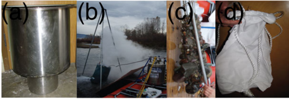
Figure 5. Field methods used to measure bed material composition and collect samples for metals analysis: (a) modified McNeil sampler; (b) tri-axial freeze core set-up with 30L nitrogen tank, boat and tripod (also see Supporting information); (c) example freeze core; and (d) hand-sewn infiltration bag. This figure is available in colour online at wileyonlinelibrary.com/journal/rra
