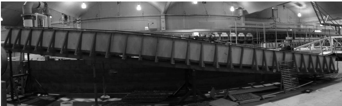
Figure 3.1. Side-view photograph of flume, at slope of 0.14 m/m. Flume length is 10 m and width is 0.6 m. Flume is straight; distortion in photograph results from photographic methods.
