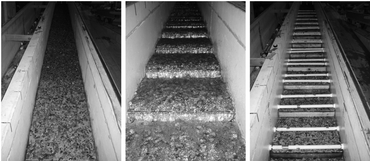
Figure 1. Flume configurations used in partitioning analysis: (left) plane bed with grains, (middle) steps with grains ( Q = 8 L/s, S = 0.14 m/m), and (right) steps with grains and LWD (high density, long-single-perpendicular configuration).
