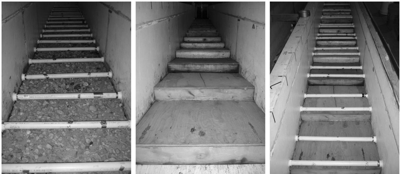
Figure 2. Flume configurations used in partitioning analysis: (left) plane bed with grains and LWD (density is high, orientation is perpendicular, and length is long), (middle) steps without grains ( S = 0.14 m/m), and (right) steps without grains, with LWD (high density, long-single-perpendicular configuration).
