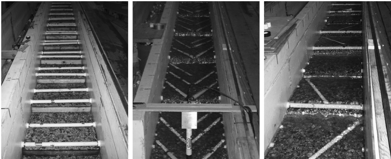
Figure 2. Upstream view of flume, showing examples of large woody debris (LWD) configurations tested to measure the effect of LWD orientation on flow resistance: (left) perpendicular (high density, S = 0.14 m/m), (middle) ramped (high density, S = 0.05 m/m), and (right) combination (medium density, S = 0.10 m/m). For all three orientations, piece length = long. Conductivity probe used for salt dilution measurements of velocity is shown in foreground of Figure 2 (middle).
