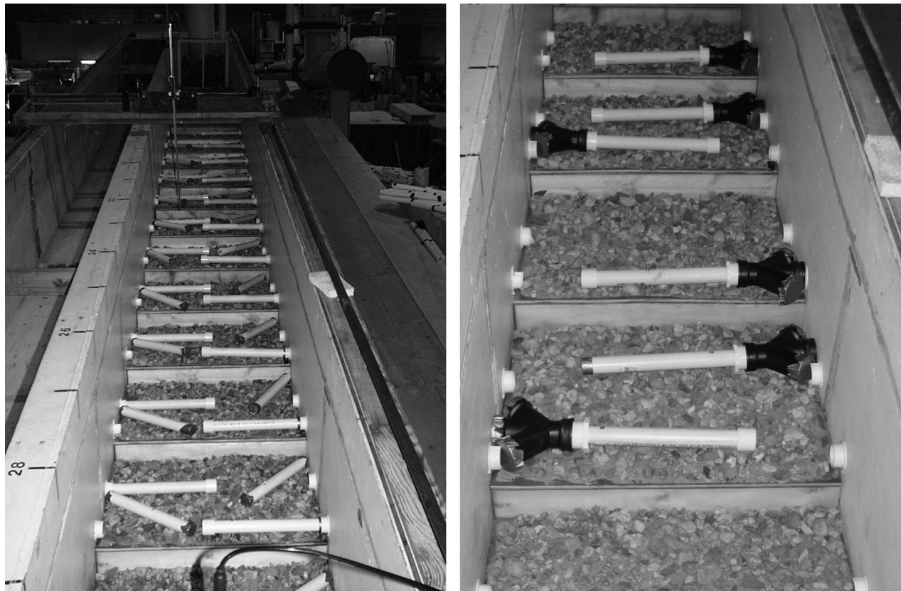
Figure 3. Upstream view of flume, showing examples of LWD configurations employed to test effects of piece length on flow resistance: (left) short pieces (high density, combination orientation) and (right) rootwad pieces (high density, perpendicular orientation). Long pieces were also tested, as shown in Figure 2.
