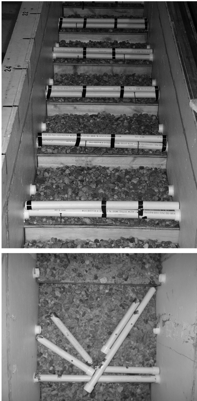
Figure 4. Two LWD arrangements assessed as part of factorial tests of the effect of LWD configuration on flow resistance: (top) stacked (high density, perpendicular) and (bottom) jams. Single pieces were also tested, as shown in Figures 2 and 3.
